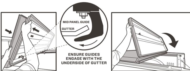
Holding mid and tail panels tightly together, begin unfolding towards tailgate.
