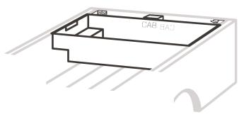
Many pickup truck cargo beds are tapered, which means that many Cross Bins have a front and back. Look for the word "CAB" etched into one of the longer walls of the bin (could be on inside or outside of wall); make that wall the one nearest the cab.
