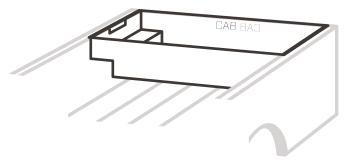
Many pickup truck cargo beds are tapered, which means that many Cross Bins have a front and back. Look for the word "CAB" etched into one of the longer walls of the bin (could be on inside or outside of wall); make that wall the one nearest the cab.
