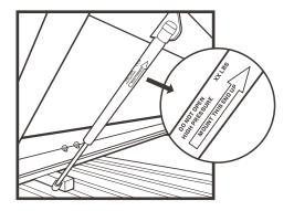
12 Attach the 2 remaining gas springs on the **tail panel**, again making sure the barrel end is up.
