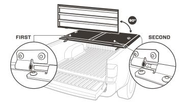
Mating hinges is easiest when you engage the longer pin first.
