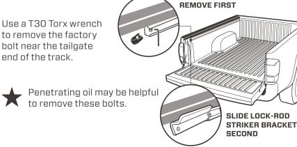
Slide the driver-side lock-rod striker bracket into the track until its forward hole aligns with the factory bolt. Reinsert the factory bolt and retighten it with the Torx wrench.
