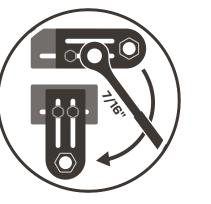
If your plastic bed rail cap extends below the metal edge of your bed rail, trim the excess at each lock rod location so that it's flush with the metal bed rail's edge.
