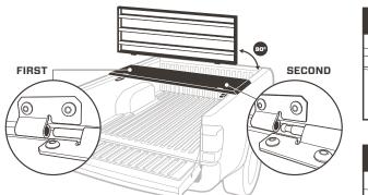
Mating hinges is easiest when you engage the longer pin first.
