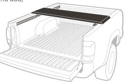
Attach the tail panel by holding it at a 90° angle from the bed rails and begin to mate the driver's side hinge first which is slightly longer.
