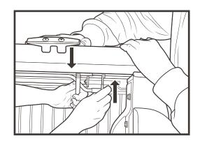
The panels may be tough to open and close at first. Leave the panels closed as much as possible to allow the weatherstrip to break in. After a few days, you'll find things working smoothly.
