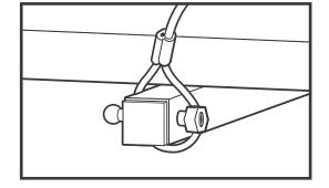
Attach 2 gas springs the cab panel.
