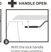
in the open position, the rod tips clear the bed rails.
