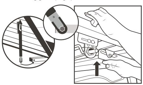
With the safety catch in place, your cab panel will only open partially. To fully open the panel, pull down on panel while using your other hand to push up on the flat part of the catch until it disengages.
