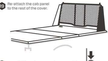
To avoid hinge damage, make sure to fully mate the hinges before bringing the cab panel back into its closed position.
