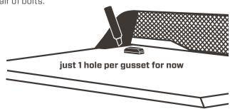
Double-check the underside of the cover to verify that nothing will obstruct the bolts or washers at these locations. Adjust the locations of the bolt holes if necessary.
